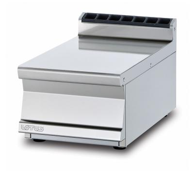
Construction - Fabricated using CrNi 18/10 AISI 304 grade Stainless Steel Scotch-Brite Satin polish Finish, incorporating 2 mm thick worktop, rounded edges, chromed details and rear splash back. Model -Professional worktop with or without drawer . Fittings - Appliance is supplied with steel or plastic tanks, h 15cm. Adjustable feet.
