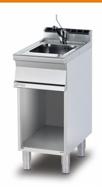
Construction - Fabricated using CrNi 18/10 AISI 304 grade Stainless Steel Scotch-Brite Satin polish Finish, incorporating 2mm thick worktop, rounded edges, chromed details and rear splash back. Model -Professional Sink with Lever arm Tap for hygiene standards on open cabinet. Fittings - Appliance is supplied with adjustable feet. Doors not Included.
