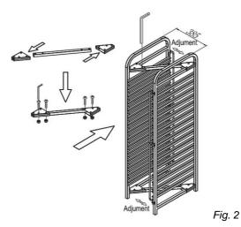
Slid the connecting strut (G) in between brackets, (B) and (C), in top part of both lateral sections (A). Fix the connecting strut (G) to the assembled brackets using 4 screws each (F) and 4 dome nuts (H), and Allen wrench (I).
