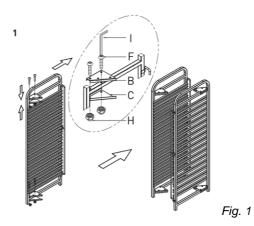
First, fix 1 bracket each, (B) and (C), at the top and bottom of both lateral sections, using 2 screws each (F) and 2 dome nuts each (H). Use Allen wrench (I) and tighten screws.
