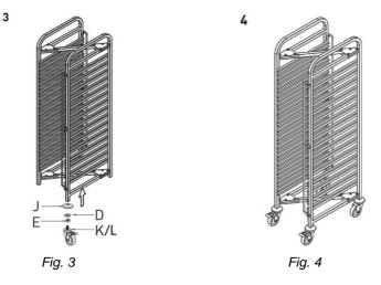
Fix 4 swivel casters, (K) and (L), on lateral sections. Place 1 nut (E), 1 washer (D), and 1 damper (J) on swivel casters and screw them into the square tubing of lateral sections (Fig. 3).
