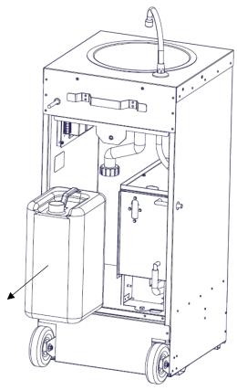
To re-install the waste-water tank, follow the above steps in reverse.
