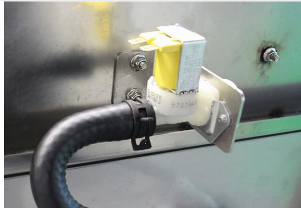
10. Secure the solenoid valve with 2 M5 safety nuts.
