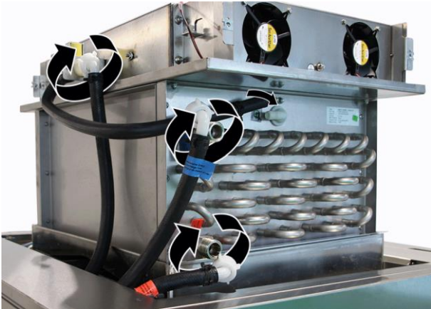
11. Connect the hoses and tighten them by hand. Secure the upper hose on the front with a spring band clamp. When fitting the hoses, pay attention to the colour markings.
