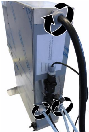
11. Tighten the hoses from the outside and attach the cover. 12. Insert the filter element and screw in the pre-filter hand-tight. 13. Hook in the pre-filter casing and push it down. 14. Screw the casing together.
