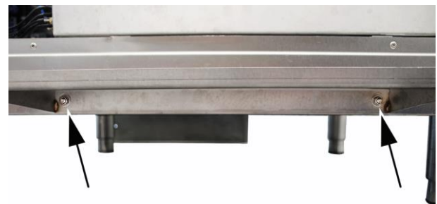
10. Insert the reinforcement profile from the inside into the base drip tray and insert the welded hexagon screws through the holes in the base drip tray.
