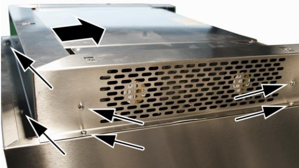
17. Push in the fan unit casing from the front. Secure the casing with 4 self-tapping screws per side and 2 self-tapping screws on the front.
